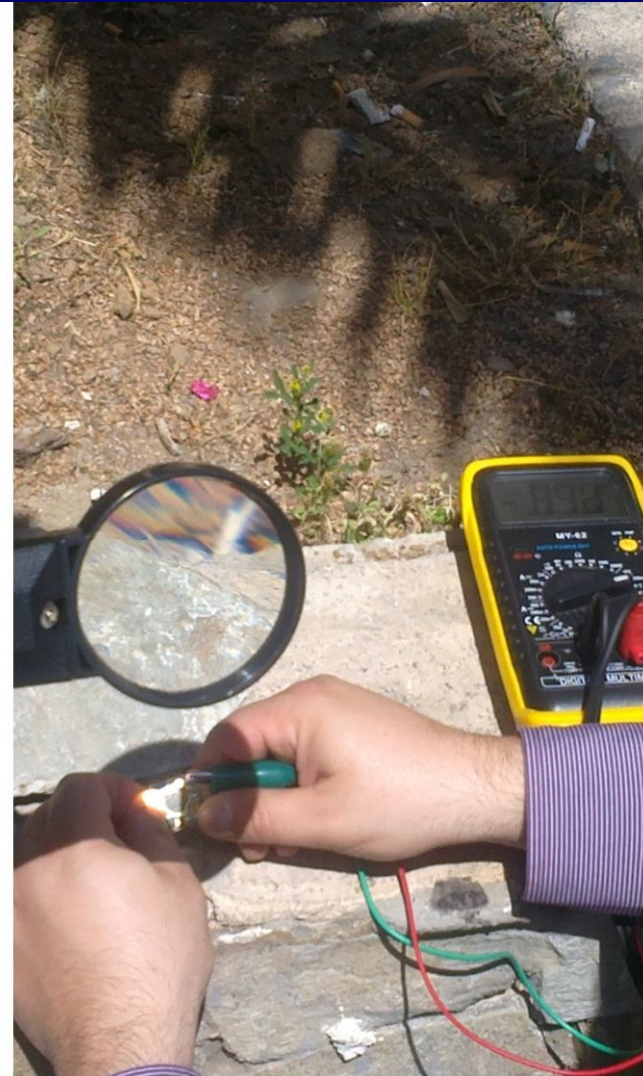
Measurement of Concentrated Cells with 80suns
